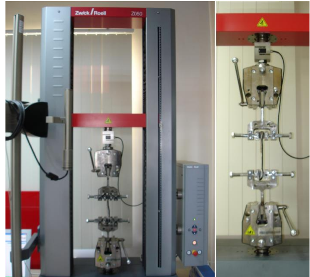
Figure 2. The tensile test setup
